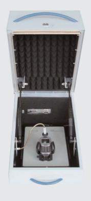
Reliable check of mobile phone's loudspeaker and microphone
